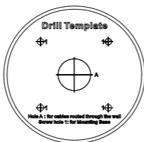
Figure 2-5 Drill Template of the Junction Box
